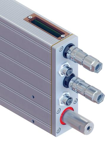
The new concept of P03 will allow the controller to be eliminated from the electrical enclosure for linear direct drives, thus greatly reducing installation time and effort. On the application side, this opens up the possibility to efficiently couple the devices in a daisy chain linkage. Modular machine concepts can also be implemented simply and easily using the new linear motors with integrated drives.
